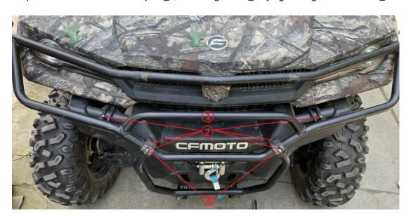
Step4: Install front upper bumper 1, mounting base 3 by tightening 4 8x20 bolts 2.
