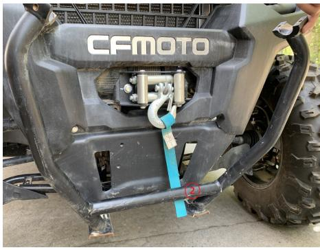
Step2: Install connecting bracket② by tightening 2 8x20 bolts①. Left side is same as right side.
