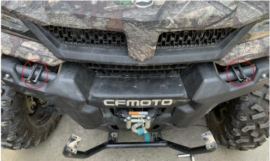
Step3: Install front middle bumper 1, mounting base 3 by tightening 6 8x20 bolts 2.
