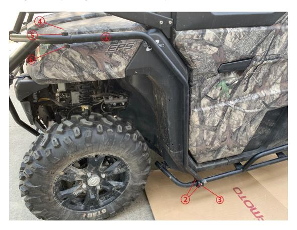
Step3: Install rear bumper ① by 2 8x25 bolts ②.
