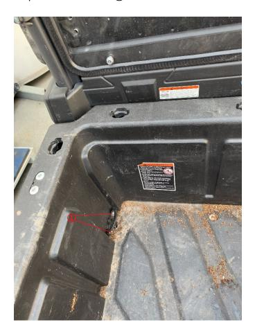
Step5: Install rear left bumper① by 8x55 bolt②, spacer bush③, barrel④ and tighten 2 bolts⑤ which have been removed in step4. Left side is same as right side.
