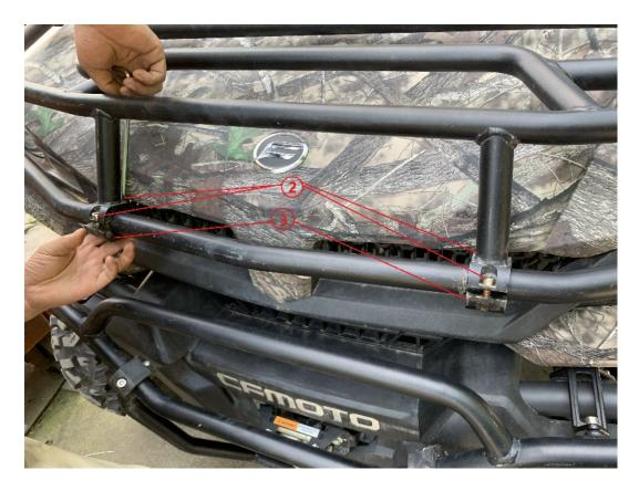
Step5: Install right mounting plate ① by tightening 2 8x45 bolts ② and 8x25 bolt ③. Left side is same as right side.
