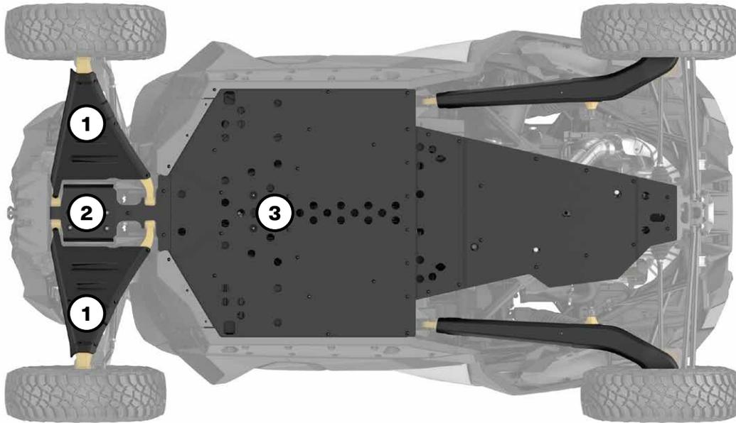
Our plastic plates glide smoothly and silently over obstacles, offering great protection in rough terrain. Made of abrasion-resistant thermoformed  $\frac{3}{8}$ " (10 mm) thick High Molecular Weight Polyethylene (HMWPE).
